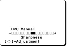
**3** While looking at the picture displayed on-screen, press the ➤ (or ≺) button, until the picture is adjusted as desired.
